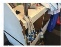
2. When you have accumulated 7 shirts on the Rope Tie Assembly Rack (Item# RA-26), reach around and grasp one Rope Tie, as shown.
