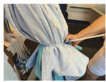
8. To remove the Rope Ties at the shirt press, grasp and press the spring-loaded buttons and pull on the button slide to loosen.
