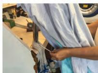
3. Bring the Rope Tie up and over the bundle of 7 shirts. Lower it to the appropriate place on the bundle, which is over the middle of the breast pocket area.
